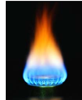
Example of improper burning gas stove.
